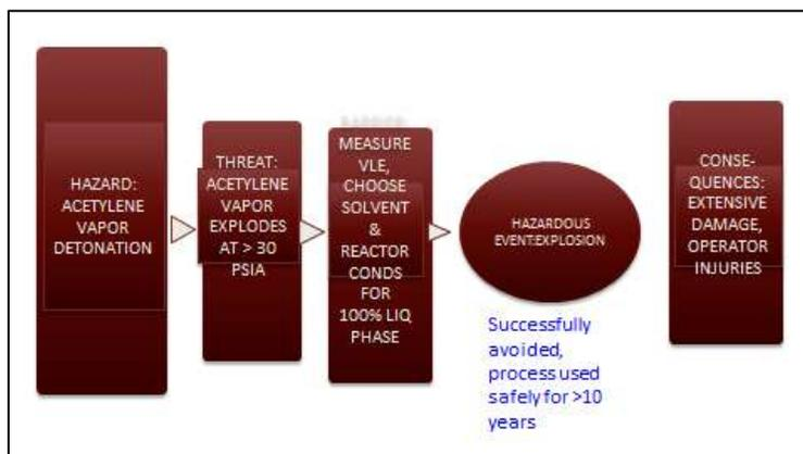
Figure 6. Bowtie Diagram – Acetylene Process Safety
