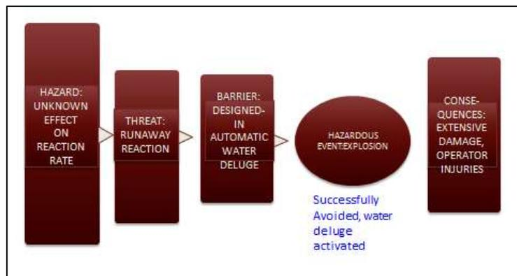
Figure 7. Bowtie Diagram – Hydrogen Peroxide Process Safety
