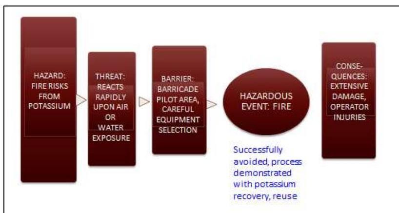
Figure 5. Bowtie Diagram – Pilot Plant Testing of Olefin Dimerization Process Safety
